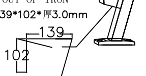
⑱ SEAT HANGING OUT OF IRON 139*102*厚3.0mm
